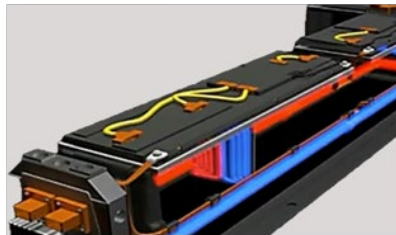
Battery Coolant Lines
